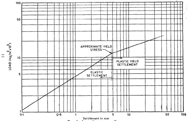
Fig. 6 Load Settlement Curve (Log-Log Scale)
