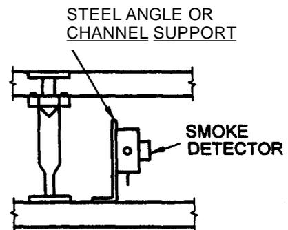
2C Above False Ceiling/Below False Floor Mounting Arrangement of Smoke Detector - Permitted
