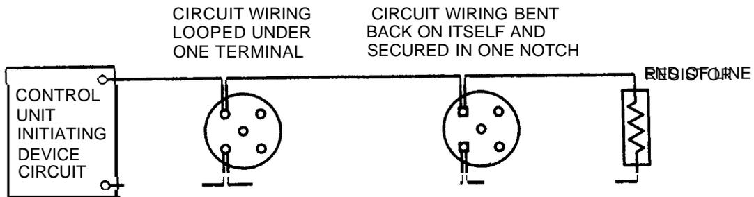
1B Incorrect Wiring Method - Two-Wire Detectors
