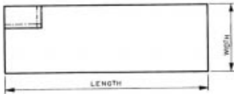
FIG. 2 RECOMMENDED LOCATION FOR TAKING TEST SAMPLES
